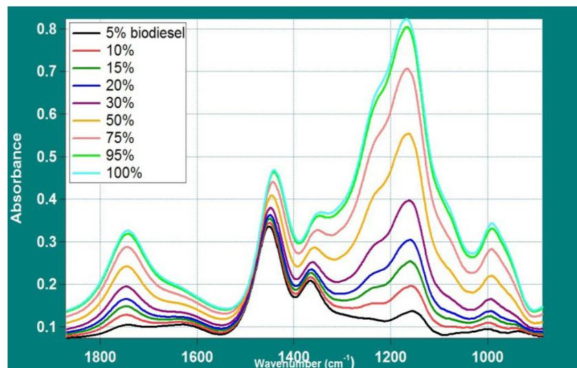
Figure 1: IR Spectra from an InfraSpec VFA-IR spectrometer of different biodiesel concentrations.
