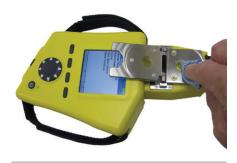
**2. Danger!** Results are flagged using a color-coded system that alerts users to out-of-specification conditions. *Courtesy: Spectro Scientific*
