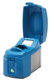
4. The split cell opens for easy cleaning. No chemicals or solvents are needed to prepare the cell for its next use. *Courtesy: Spectro Scientific*
